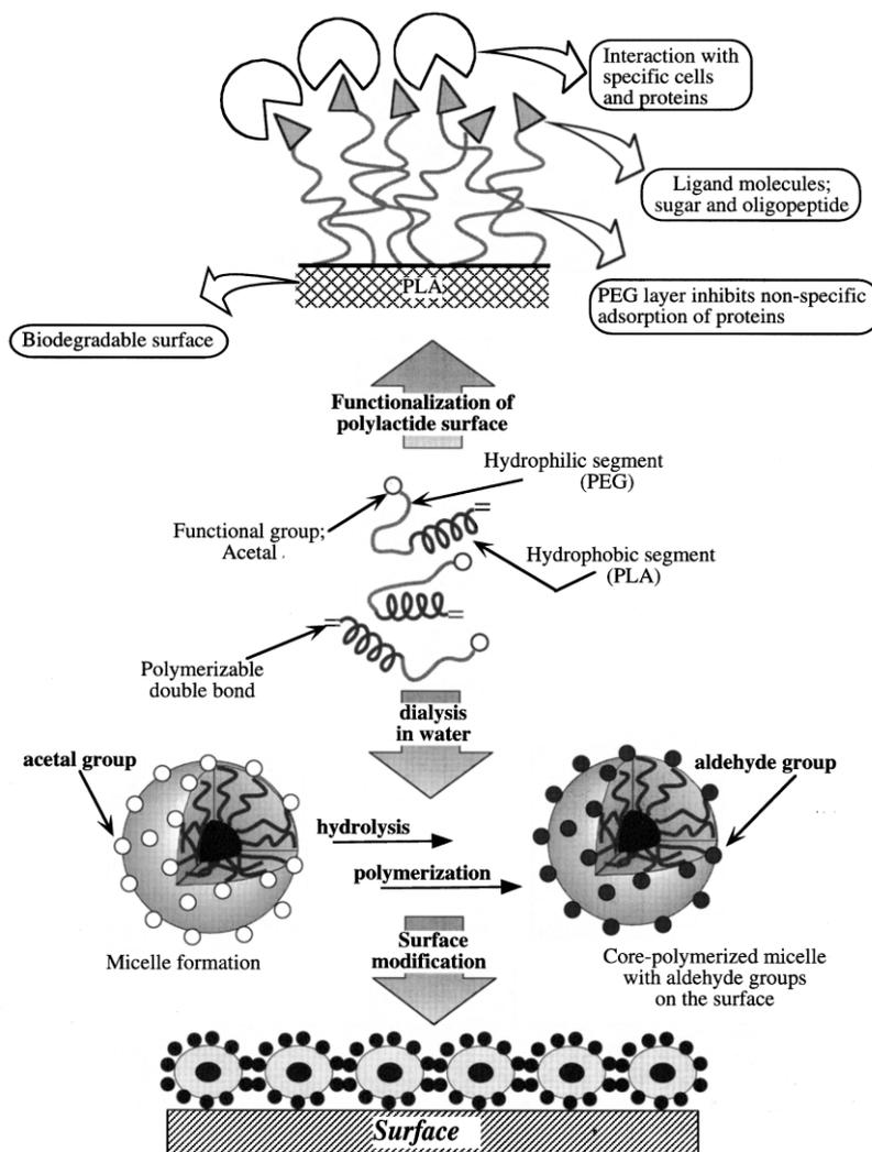
Fig. 1. Schematic representation of the application of heterobifunctional PEG-PLA block copolymer for the construction of functional PEG layer at the materials interface.
