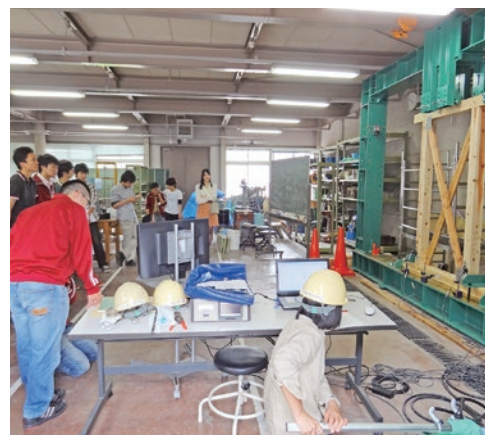
■木造軸組の構造実験 A Structural Experiment of Wooden Frame
