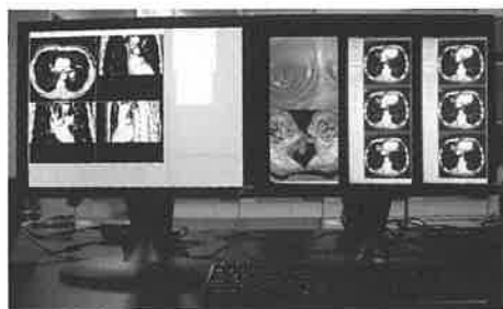
Figure 9. Two black-and-white high resolution liquid crystal display monitors (Computer-aided chest diagnosis workstation)
