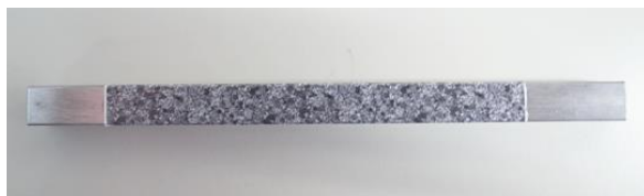
Fig.4 A specimen painted the random pattern for the DIC method
