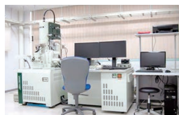
電界放出形走査電子顕微鏡 (FE-SEM) Field Emission Scanning Electron Microscope
